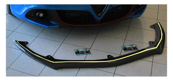
APPLY ACTIVATOR PRIMER ON THE AREA HIGHLIGHTED ON THE FRONT LIP, AS WELL AS ON THE BUMPER AREA WHERE THE GLUE WILL BOND.
